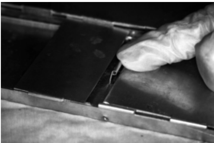
Figure 4. Trigger mechanism of Sherman ® live-capture trap, showing "catch" that holds front door of trap open. Push the catch back as shown to increase sensitivity of the trap. To decrease sensitivity, place finger behind catch and pull forward.
